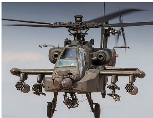
The Boeing AH-64 Apache is an American twin-turboshaft attack helicopter
