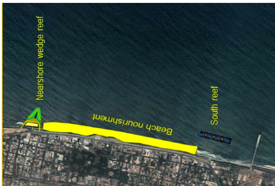
Figure 1 - Beach Stabilization with artificial reefs
