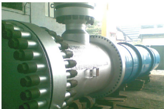
101/CA Tube-in-Tube, Waste Heat Reboiler – my first major order
