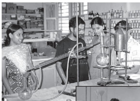
➤ The Soxhlet Extractor — an apparatus used for extracting various types of oils.
